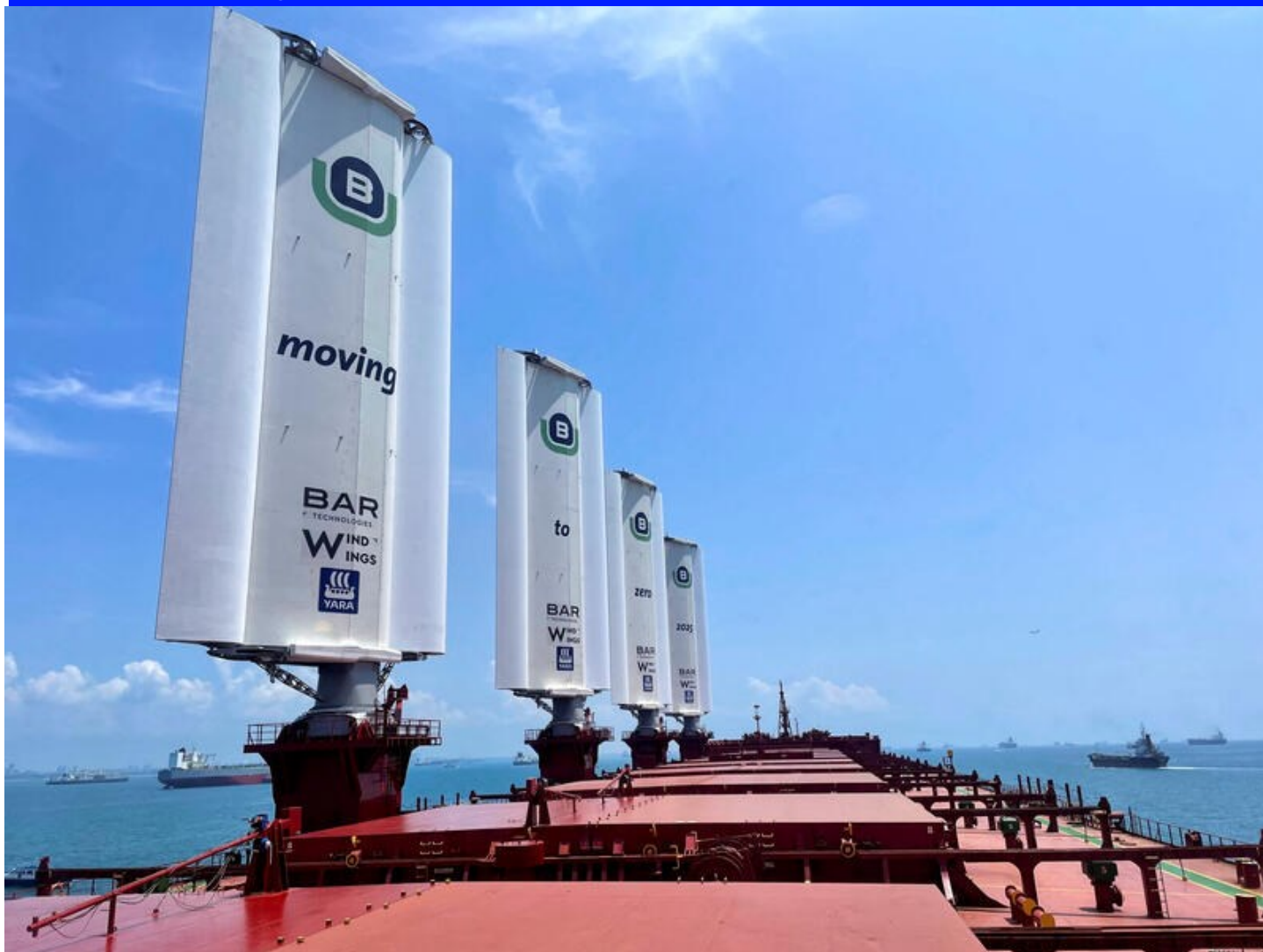
A view of the four WindWings as seen onboard bulker ship Berge Olympus, in Singapore October 12, 2023. REUTERS/Jeslyn Lerh
