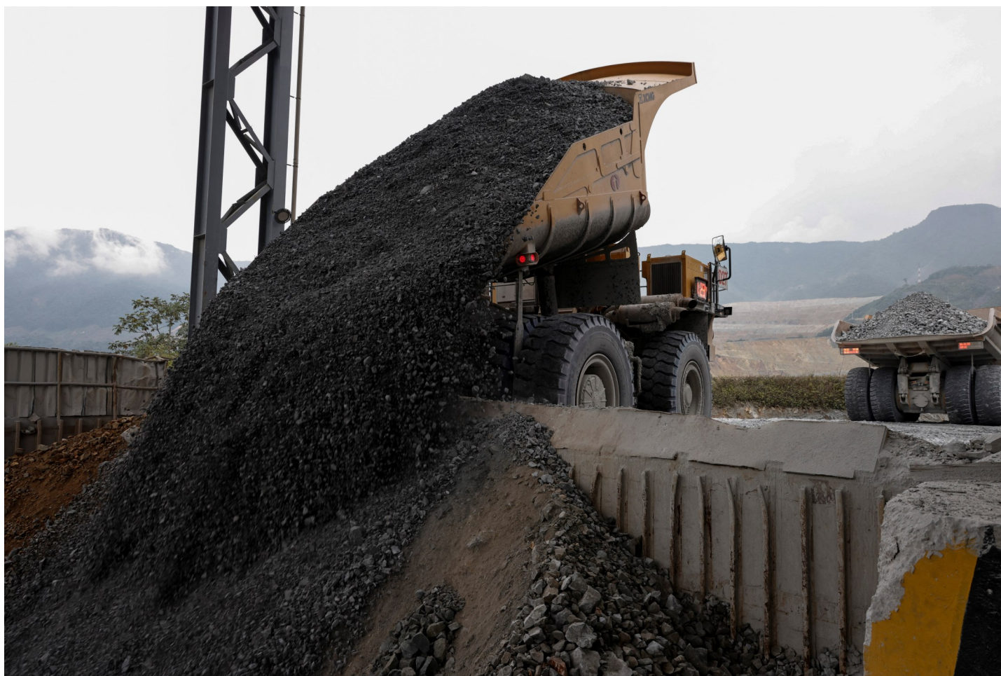
A dumper deposits material in the primary crusher, where minerals are separated from waste materials, at the Mirador Mine, in Tundayme, Ecuador, August 15. REUTERS/Karen Toro
