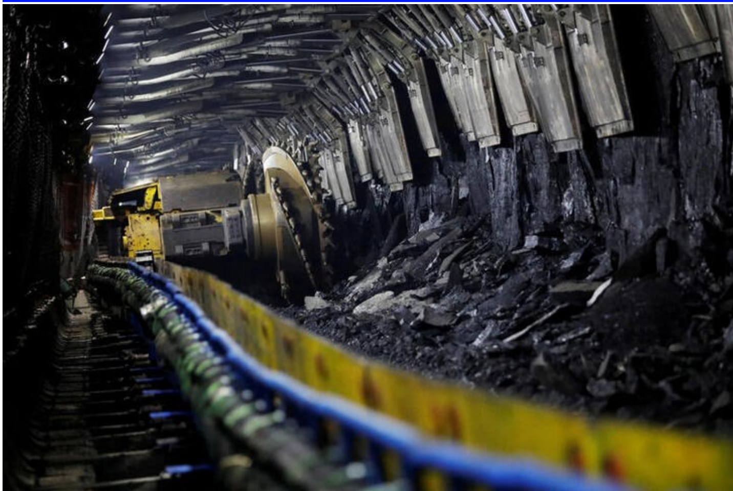
A shearer is pictured at an underground coalface where Huawei 5G base stations are deployed to support communication and remote control, at Xiaobaodang Coal Mine, during a Huawei-organised media tour, in Shenmu of Yulin city, Shaanxi province, China, April 26. REUTERS/Tingshu Wang
