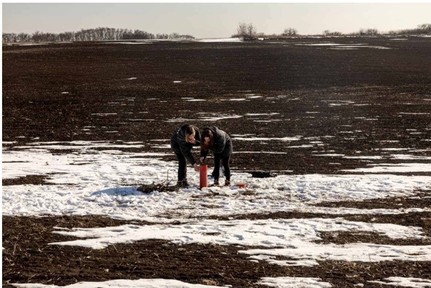
Environmental experts of CDM Engineering Ukraine, Yuliia Zazerina and Alina Tatarchuk test the groundwater level at the Polokhivske lithium deposit that will be developed by Ukrilithium Mining in the Malovyskivsky district of Ukraine's Kirovograd region, amid Russia's attack on Ukraine, February 27. REUTERS/Thomas Peter
